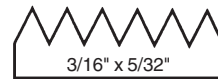
3/16" x 5/32" V Notch 3 ply and 5 ply Engineered Plank Coverage: 50 sq. ft. per Gallon
